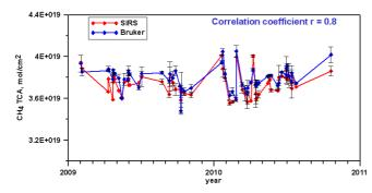
Fig.4 Results of simultaneous measurements of CH4 TCA.
